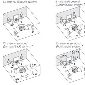
a. This layout is available only when the additional amplifier is connected to the unit and the surround back or front height speakers are connected to the amplifier. For details, see Connect the surround back or front height speakers on page 11.
